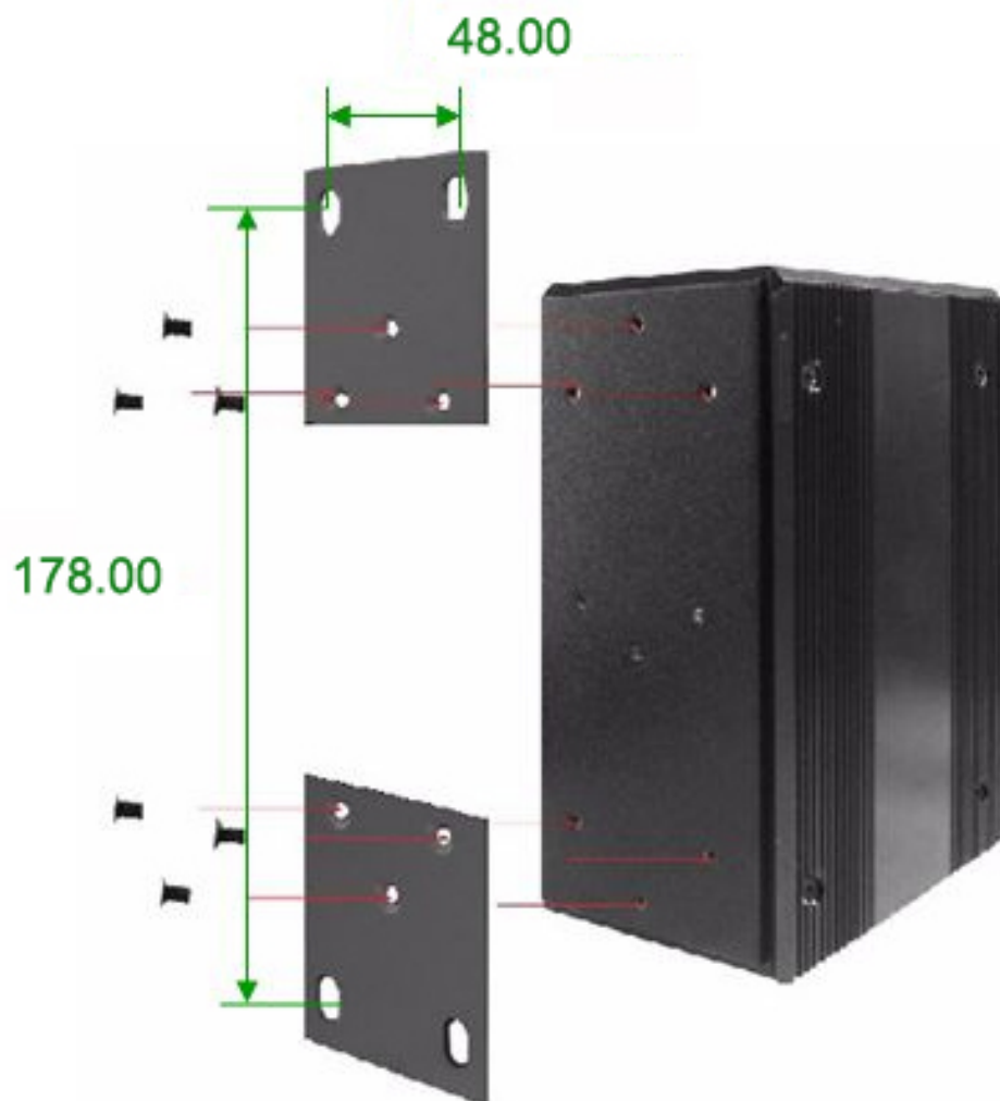
Figure 2.5: Combine the Metal Mounting Kit (units: mm)
